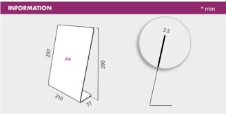
This Sign Holder Display has a "L" shape and it features an A4 format mirror 2.5mm thickness surface, which can be labelled with logos or graphics. This display is ideal for being used in optical shops, jewelers or hairdresser where customer can get a unique and custom last impression.
