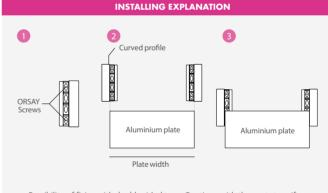
Possibility of fixing with double sided tape. Continue with the next steps if you wish to screw it to the wall:
