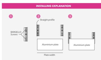
Possibility of fixing with double sided tape. Continue with the next steps if you wish to screw it to the wall:
